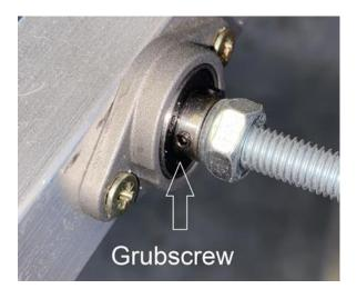
You are done with assembly. Check that the arm rotates freely.
