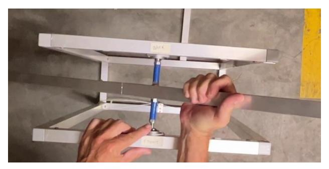
The threaded rod should be even with the outside of the bearing. The target should be facing the front where the cord is secured, for easy operation.
