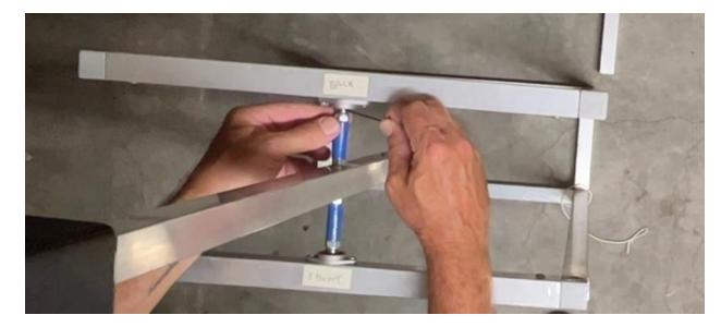
Secure in position with the 2 grub screws on each side.
